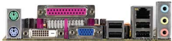
Back Panel I/O Ports
